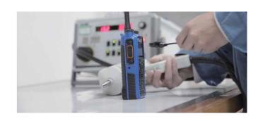
Hytera applies patent on electrostatic free design and dualmaterial molding technology in this intrinsically safe portable. The static dispersive material (blue) minimizes static accumulation on the surface, thus reducing the probability of static discharge on the radio. Meanwhile the robust material (black) maximizes the ruggedness of the enclosure.
