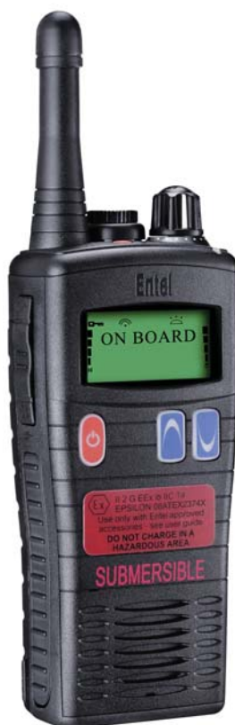
Pictured: UHF ATEX variant with stubby antenna
